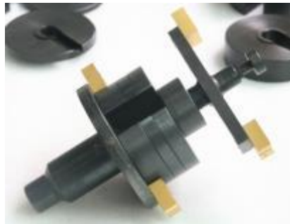
Basic Hammer equipped with weight sets to meet different impact energy
