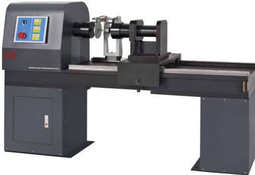
This series torsion testing machine is mainly used for performing torsion test on metal, nonmetal and compound materials complying with international standards. We offer various models to cover torsion test from 500Nm to 3000Nm.
